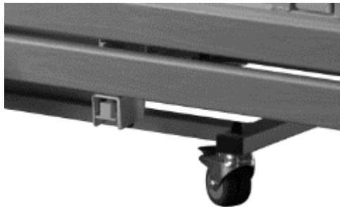
Figure 14: Pressed pushbutton/limit switch through lowered side rail
