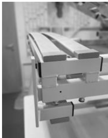
Figure 10: Assembly of the foot traverse (200 cm lying surface length)
