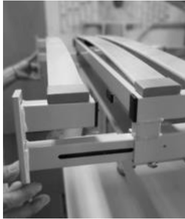
Figure 12: Assembly of the foot traverse (220 cm lying surface length)
