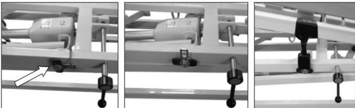
Figure 20: Procedure for securing the lying surface against folding up
