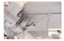
The mattress base can be turned in and out manually using the emergency release on the rotary motor.
