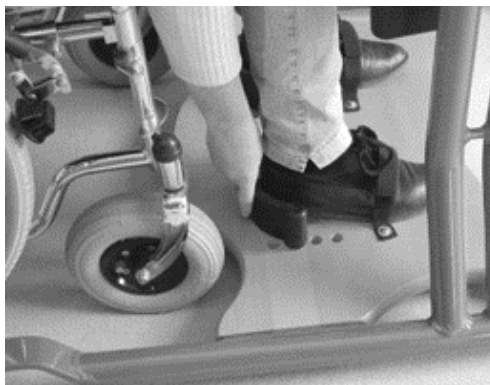
Figure 5: Adjustment of heel cups and toe fixation
