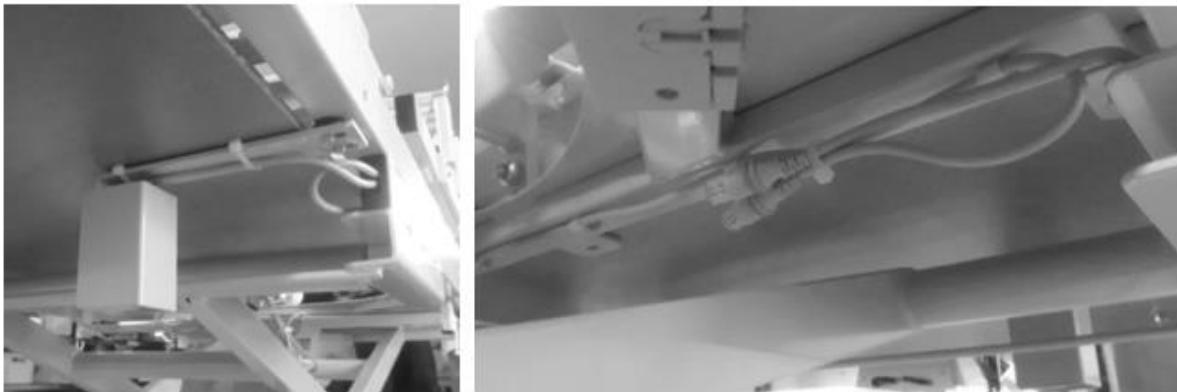
Figure 16: Mounting method of the limit switches at the mounting frame or 14 cm thick mattress
