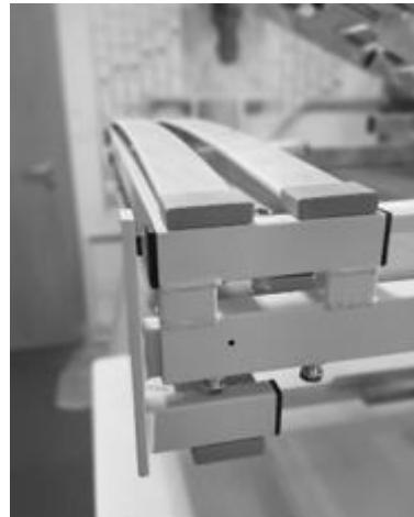
Figure 10: Assembly of the foot traverse (200 cm lying surface length)
