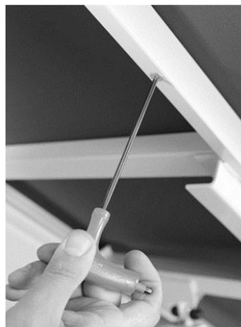
Figure 2: Unscrewing the lying surface
